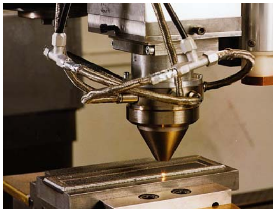
Fig. 4 Coaxial powder nozzle for laser welding experiments
