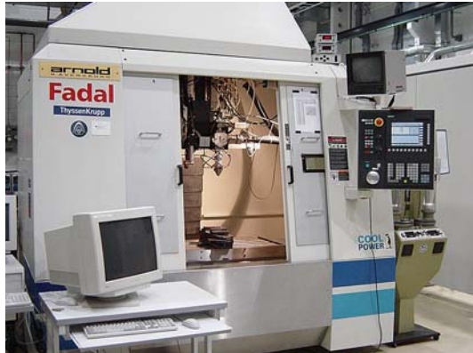
Fig. 3 Automated system for laser welding experiments
